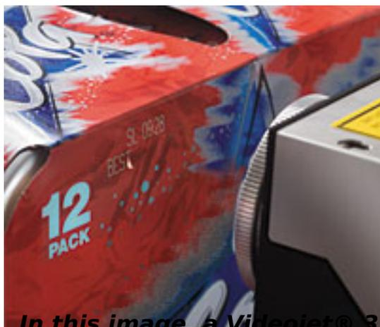
***In this image, a Videojet® 8120 10-watt laser coder is removing ink from a 12-pack carton of soft drinks, a process known as ablation.***
