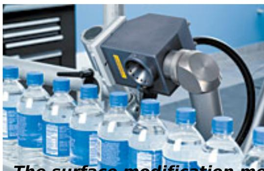
***The surface modification method of laser coding melts or alters the surface of a product or package in order to create the code. It's extremely***
