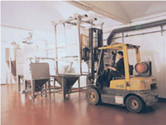
An automated product transfer system consisting of a bulk bag unloader and flexible screw conveyors tripled output of Drywite Ltd.'s dry ingredient for treating cut potatoes for mass consumption of fish and chips. The system allows the British company to satisfy growing worldwide demand for its 'Drywite' product, which preserves the cut potato prior to frying for a better and fresher presentation with less absorption of fat.
