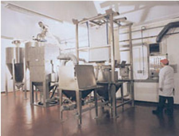
For operation under a low ceiling, the bulk bag discharger frame splits into three sections consisting of cruciform, intermediate frame and base frame. A forklift loads the cruciform with suspended bulk bag onto the intermediate frame at floor level remote from the base frame. The intermediate frame, with bulk bag in place, is maneuvered between two ceiling members and, with minimal clearance to the ceiling, is then lifted onto the base.
